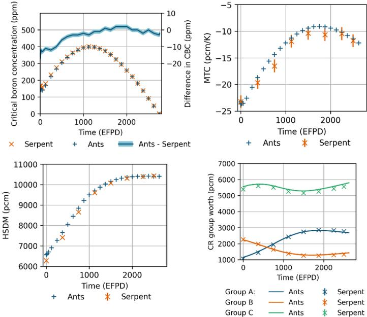
*Automatic evaluation of licensing relevant data during the simulation of an SMR operating cycle. Verification by switching one physics from reduced order solver (Ants) to a high-fidelity one (Serpent), while Kharon and SuperFINIX models are kept constant*
