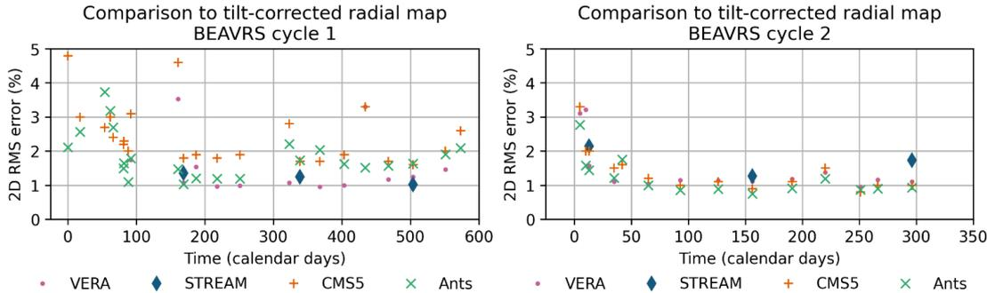
*Validation:* 2D RMS errors when comparing calculated results to measured detector maps during the two operating cycles of the BEAVRS benchmark. Various industry and scientific leaders and Kraken (Ants).
