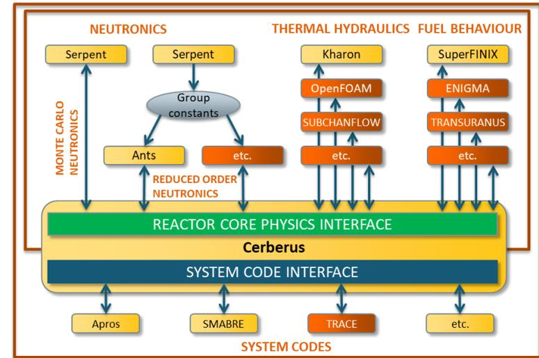
A schematic representation of the plans for the completed Kraken framework. Finnish solver modules developed at VTT are shown in yellow, while potential state-of-the-art third party solvers to be coupled are shown in orange.
