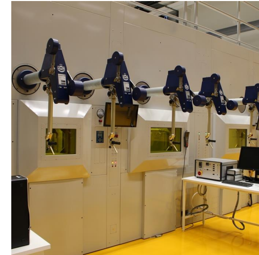
The new VTT Centre for Nuclear Safety has hot cells for research and testing of radioactive structural materials from nuclear power plants.
