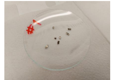
Picture T1.2. Sub-samples of highly activated steel samples ready for DTM analyses
