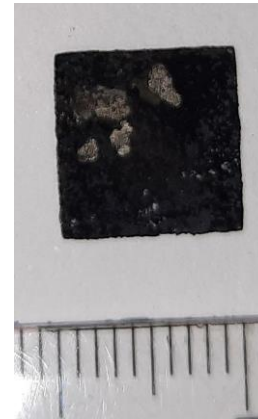
Irradiated and leached steel sample (1 cm x 1 cm)
