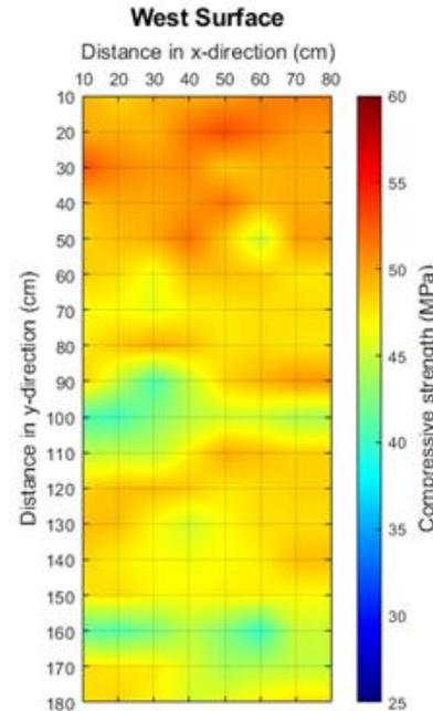
*Compressive strength values by combining the results of the UPV and rebound hammer measurements*
